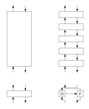
Figure 4: Hierarchical decomposition of the vaporliquid equilibrium cascade into a cascade of stages, then the decomposition of a stage into a mixer M and a flash unit F.
