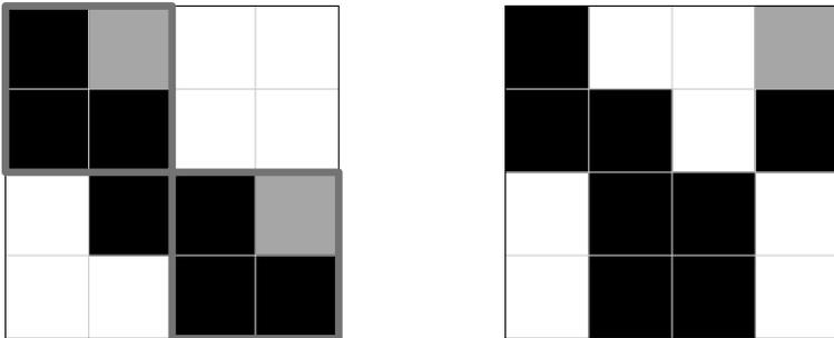
FIG. 5. Left: Performing block lower triangular decomposition first, and then applying tearing to the two  $2 \times 2$  blocks on the diagonal leads to suboptimal results. The variables that have to be guessed in each block are marked in gray. Right: The optimal ordering. The only guessed variable is marked in gray.
